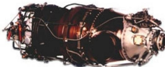
The ATR 72-200 utilizes two 1610kW (2160shp) Pratt & Whitney PW-124B turboprop engines; the ATR 72-210 utilizes two 1950kW (2480shp) Pratt & Whitney PW-127 turboprop engines; and the ATR 72-500 utilizes two 2051 (2750shp) Pratt & Whitney PW-127F turboprop engines. In its fifteen years of evolution, the PW100 family has been developed in a number of different models, generating 1,800 shaft horse power (shp), to over 5,000 horsepower in the PW150.
